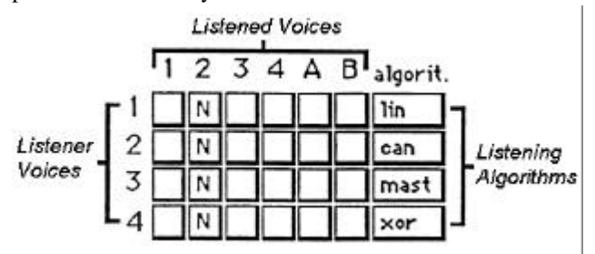
Figure 1. PITEL listening matrix. In this configuration, all four internal voices are listening to voice #2 (although using different algorithms), creating a slightly homophonic effect. Voices A and B correspond to the human players.
