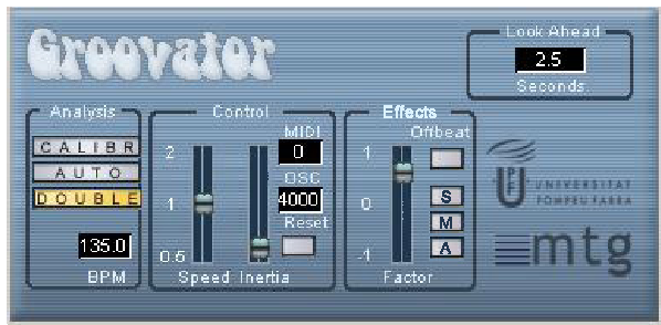
Fig. 1: Groovator's user interface for the streaming implementation. It is divided in three sections: Analysis, Control and Effects. On top, use set the look-ahead buffer size in seconds.
