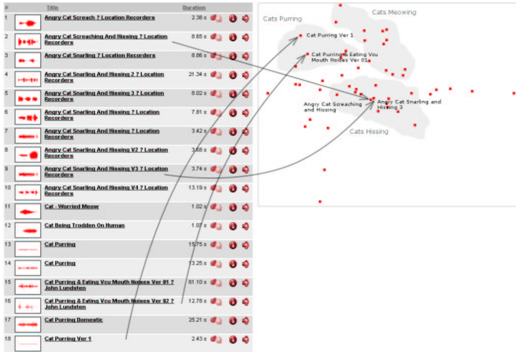
Figure 6: FastMap visualization screenshot. The points of the 2D map refer to different audio samples. The distances on the euclidean space try to preserve distances in the hyper-dimensional perceptual space defined by the similarity distance of subsection 4.1
