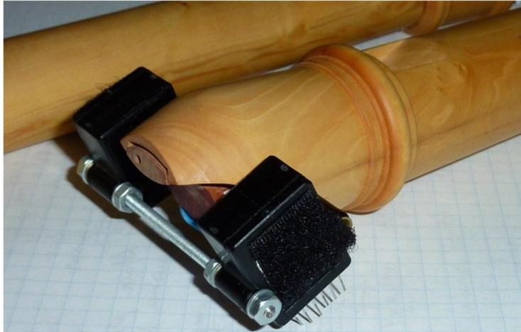
Figure 21: Prototype of recorder with pressure sensors mounted
