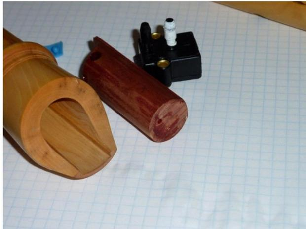
*Figure 67: View of the mouthpiece, the bloc and one of the sensors (photo from Josep Tubau)*
