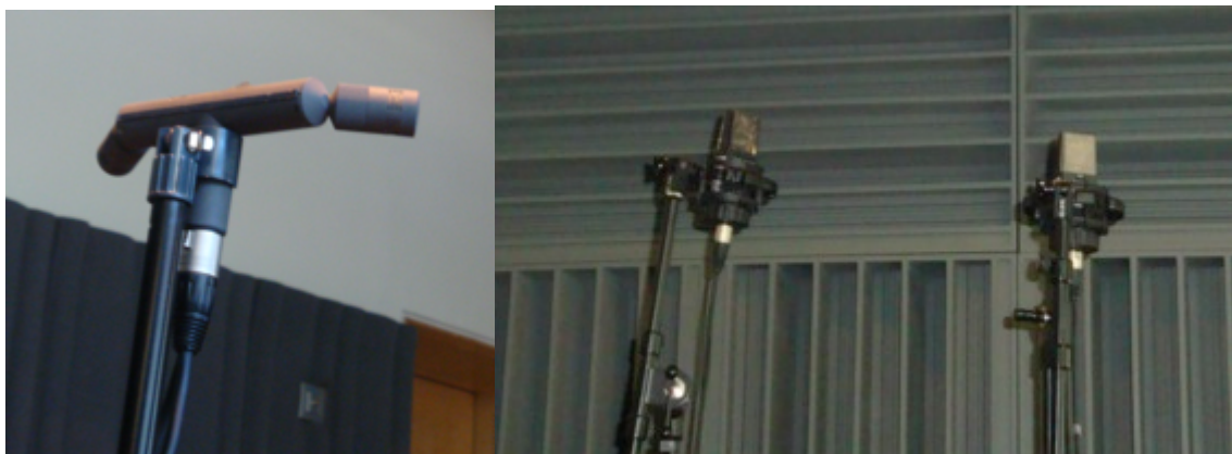
Figure 12: Microphone techniques used. ORTF (left) and AB (right)
