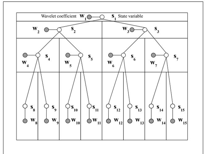
Figure 2: Hidden Markov tree model. Associated with each wavelet coefficient at a certain position in the tree structure (black node) is a hidden state variable (white node), that indexes into a family of parametric distributions.
