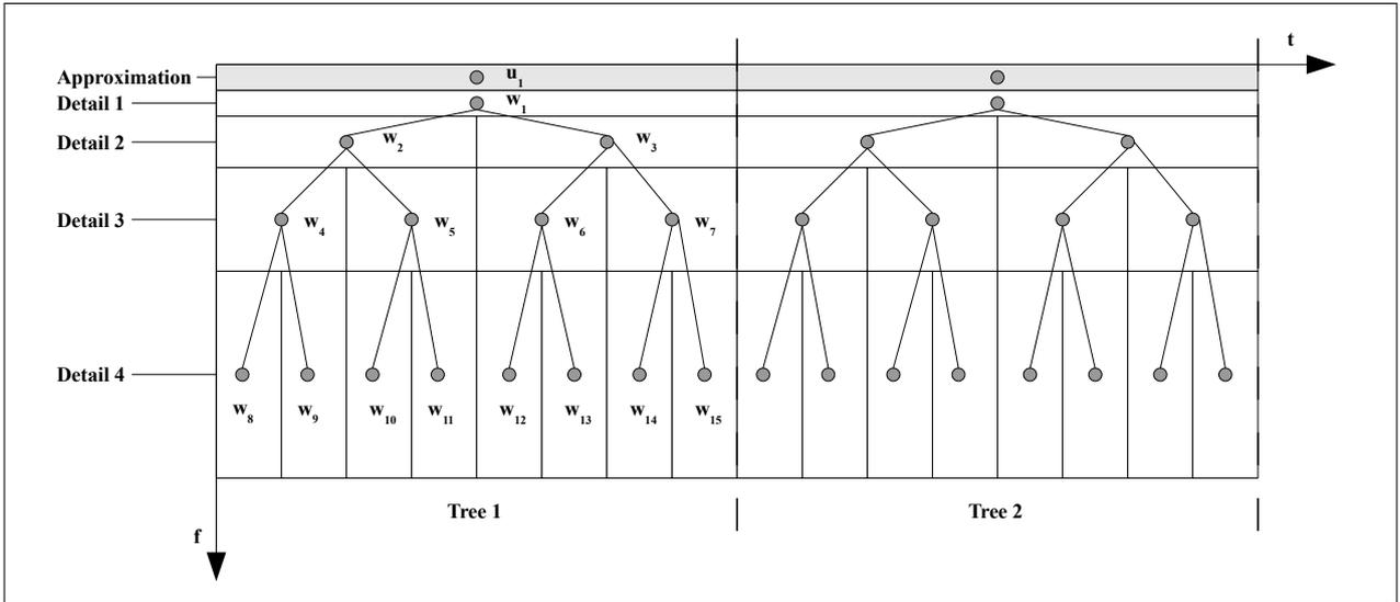
Figure 1: Four level wavelet time-frequency decomposition. Shown are two consecutive trees with frequency running downward and time to the right.
